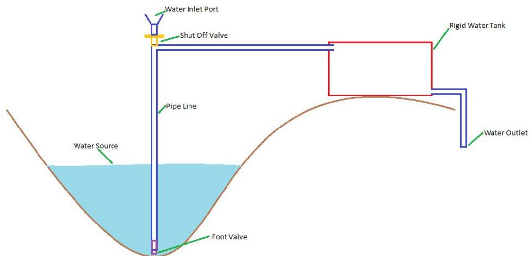
Shown in the picture above, there is a rigid water tank made from metal or concrete where it must be able to withstand implosion. Depending on total water displacement inside the tank the implosion will be great and can damage the tank if it is not able to withstand it.
