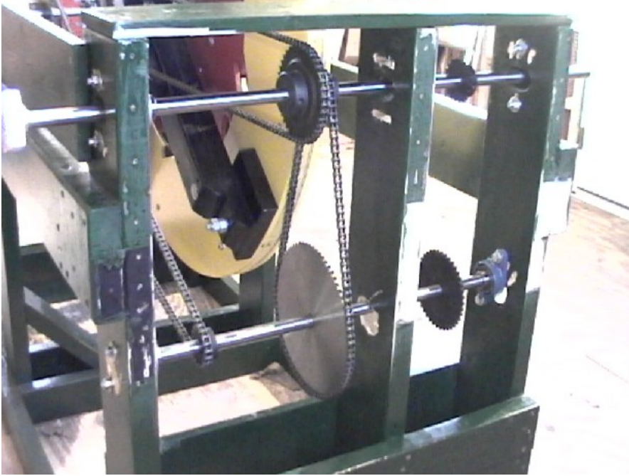
Preston Stroud Side View with Gearing & Jack Shaft Chains of BuzzSaw Gravity Wheel
