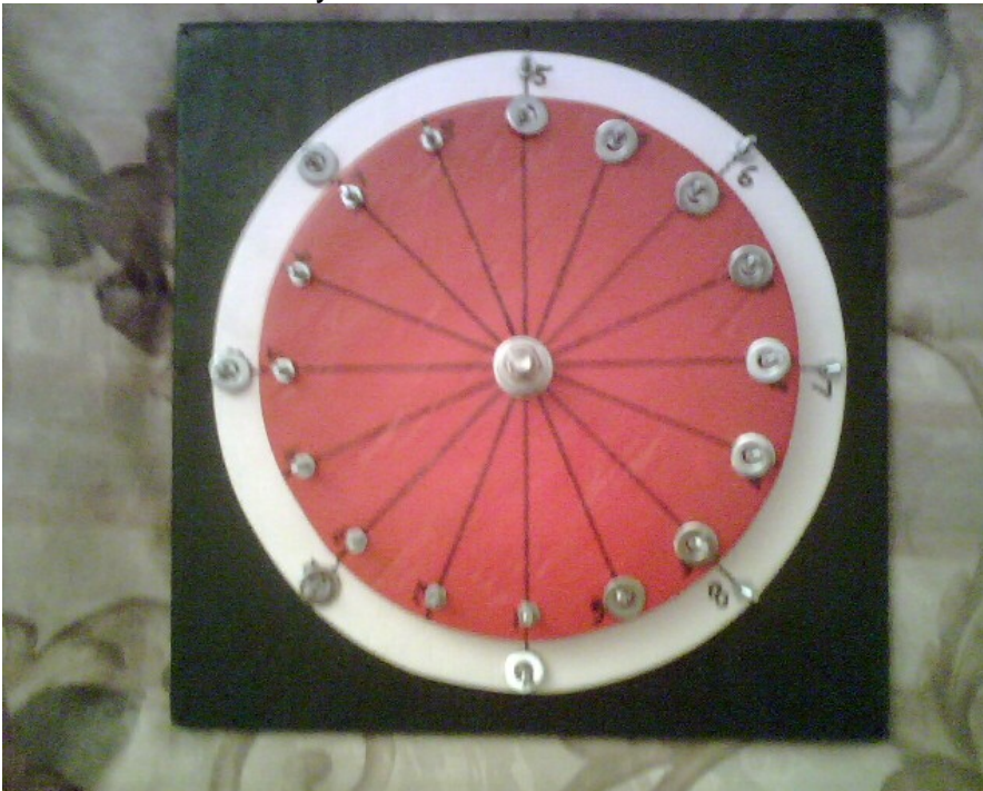
Preston Stroud Toy Test Model for evaluating concepts of gear ratio and weight patterns on the BuzzSaw Gravity Wheel
