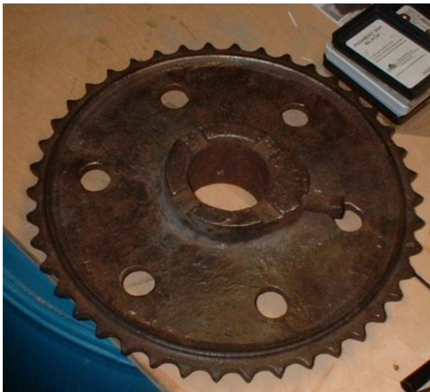
42 Tooth Custom Sprocket that came With the wheel; attached to the yellow wheel
