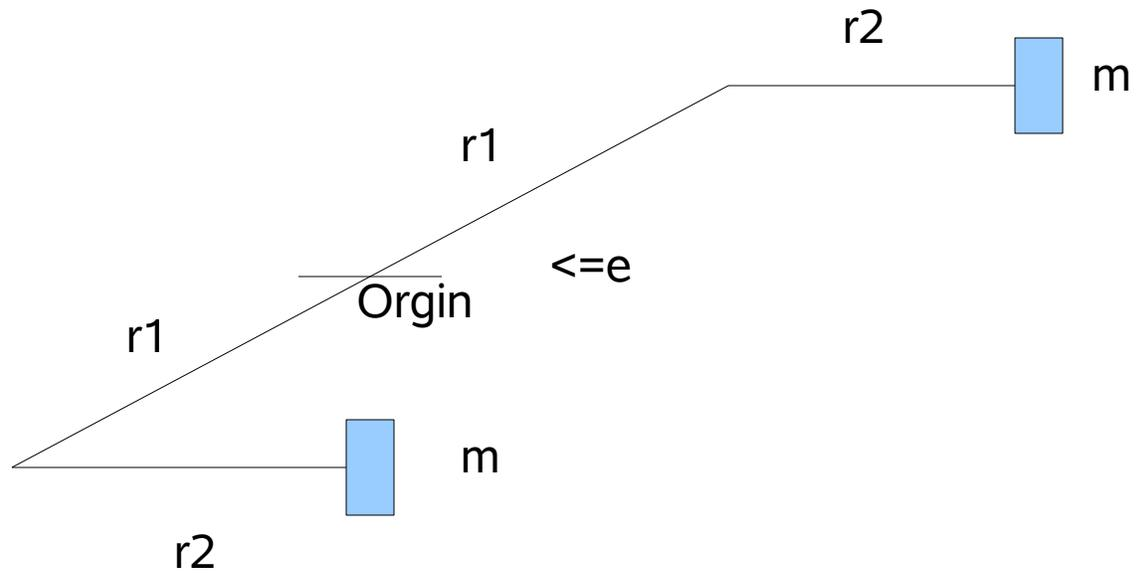
Torque Left must equal torque right for unit NOT to work, hence:
